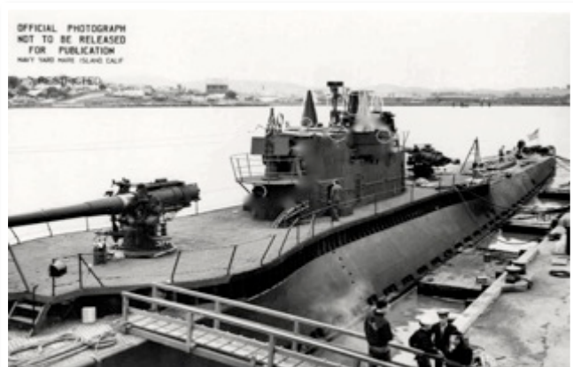
U.S.S. Narwhal (SS-167), launched on 17 December 1928 at Portsmouth Naval Shipyard, had a displacement of 2,730 long tons, a length overall of 371 feet and beam of 33 feet. In 1943, she carried a compliment of 9 officers and 80 enlisted men. She had a range 9,400 nautical miles at a surface speed of 10 knots, and her test depth was 300 feet. Narwhal participated in the Battle of Midway and saw action in the Aleutian Islands before being tasked to Spyron. From October 1943 to September 1944, during six patrols, Narwhal evacuated 128 civilians from the Philippine Islands; she earned 15 battle stars for service during the war, making her one of the most decorated ships in the U.S. Navy. Another highly decorated submarine, Narwhal's sister ship, the U.S.S. Nautilus (SS-168), and a number of other submarines assigned to Spyron also carried out missions to supply the guerillas and evacuate civilians. From December 1942 to January 1945 there were 58 such missions.
